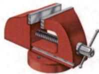
Vise — A vise does much of the same job as a wood clamp. The main difference is that it is mounted to a workbench.
