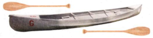
Like all boats, the front of a canoe is called the bow. It is identified by the distance the seat is positioned from the front of the boat, allowing for leg room. The back of the canoe is called the stern. The seat is positioned closer to the back of the boat since your legs will be toward the middle of the canoe.
