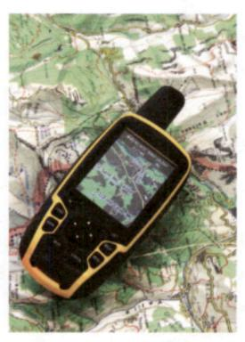
The Global Positioning System, known as GPS, is a satellitebased radio navigation system owned and operated by the United States government.
