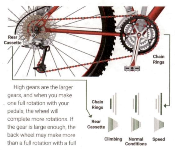
rotation of your pedal. This would mean when you pedal once, the back tire will go around more than once. This makes it harder to pedal. High gears are used when you want to go fast on flat areas or when you're going downhill.
