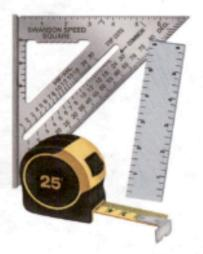
Tape measure — A tape measure lets you accurately measure pieces of wood up to several feet long. A 12- or 16-foot retractable tape measure will handle most jobs around the home. Most retract automatically and have a locking mechanism to keep the tape from recoiling (rolling up inside the case) before you're ready.
