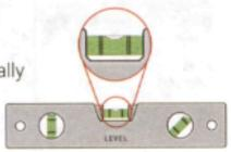
To check to see if something is level, we use a tool called a level. There are several different types of levels, but they all have a small tube of colored water that has a bubble in it. When the level is placed on a flat surface, the bubble will be in the center of the tube. If something is not level, the bubble will float to the side that is too high.
